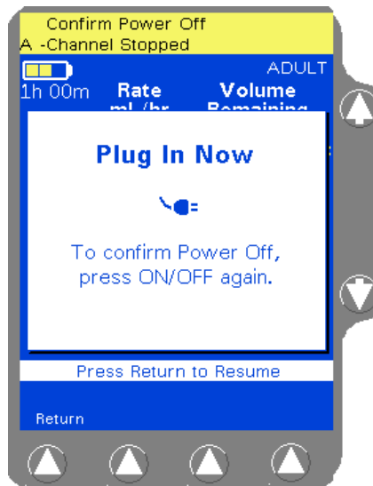
Power Off Pop-up on Battery Power
