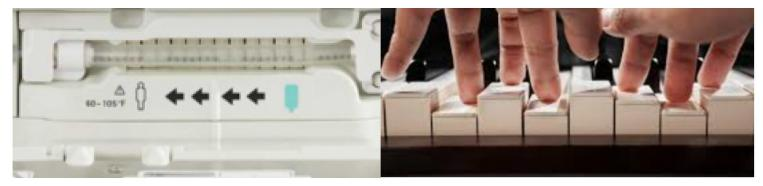
Behind the tubing are mechanical fingers (Peristaltic Fingers) that move in and out against the door plate at different rates or rhythms to move fluid forward. At least one finger is touching the door plate at any given time and this is one of the features that prevent free flow.
