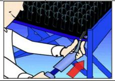
STEP 2 Slide the pump's rubber nozzle over the valve and inflate the cushion until it begins to slightly arch upward.
